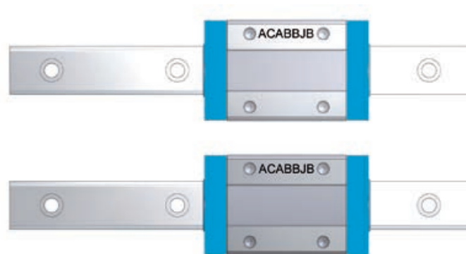
Figure 3.4 Marking the main and auxiliary guide
